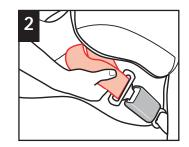
Grasp both vehicle belts together just behind the latch plate and unbuckle. **NOTE:** If the latch plate ends up behind the child restraint, grasp the belts to the outside of the child restraint, as close to the latch plate as possible.
